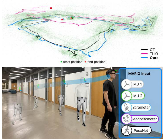
Figure 1. We propose MARIO, an inertial odometry framework that builds on a single-IMU model, grounds motion in lower-body pose predicted by a pretrained PoseNet, and enhances robustness through sensor fusion with a secondary IMU, barometer, and magnetometer.
